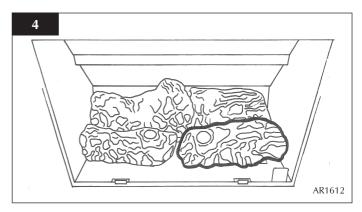
7.4 Place log D across from the rear log A to log B on the lefthand side. There are cut-outs in both logs for location. See diagram 5.
